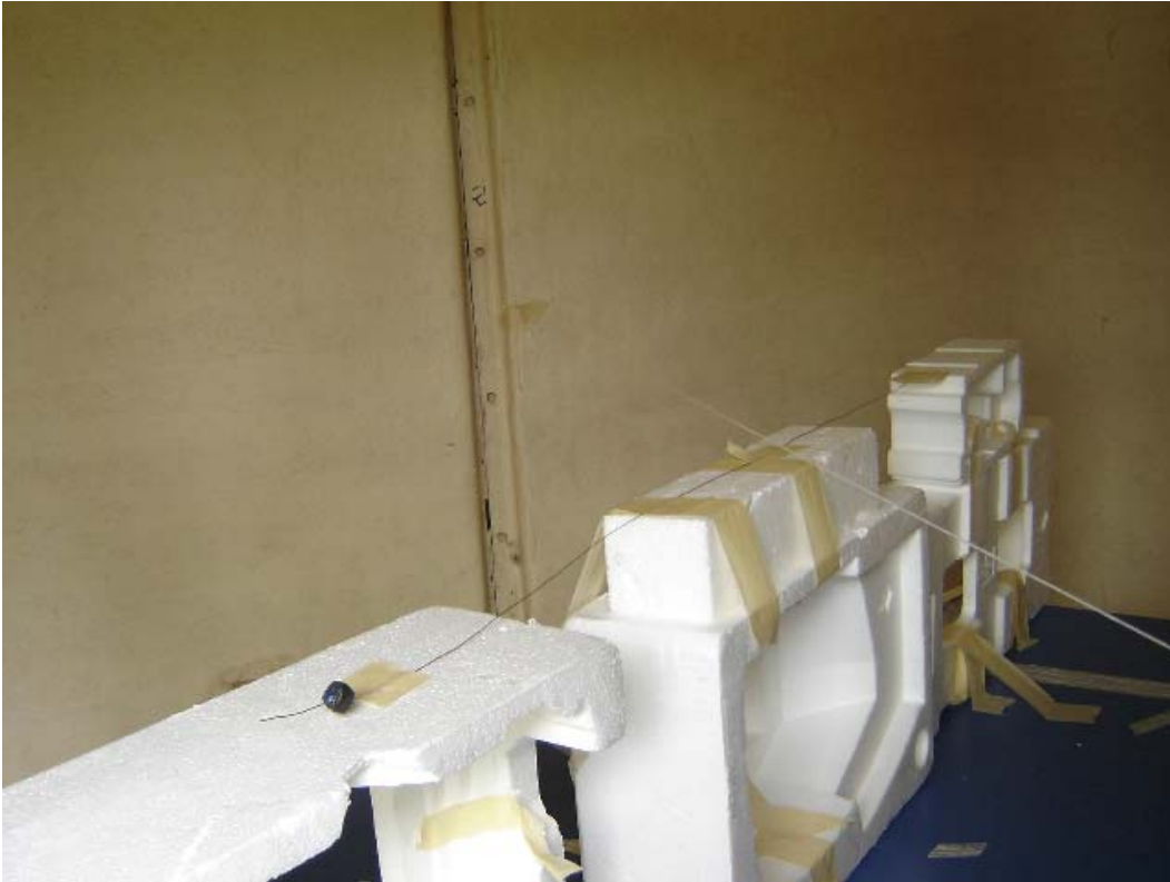
Photo 1. Wire and 0.15m section on the turntable.
